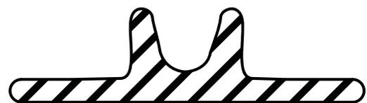
The unique dual rib profile optimizes rigidity & stability while still maintaining a degree of flexibility. This design, unique to Quantum provides for easy center drilling & attachment of optional signs and hardware.
