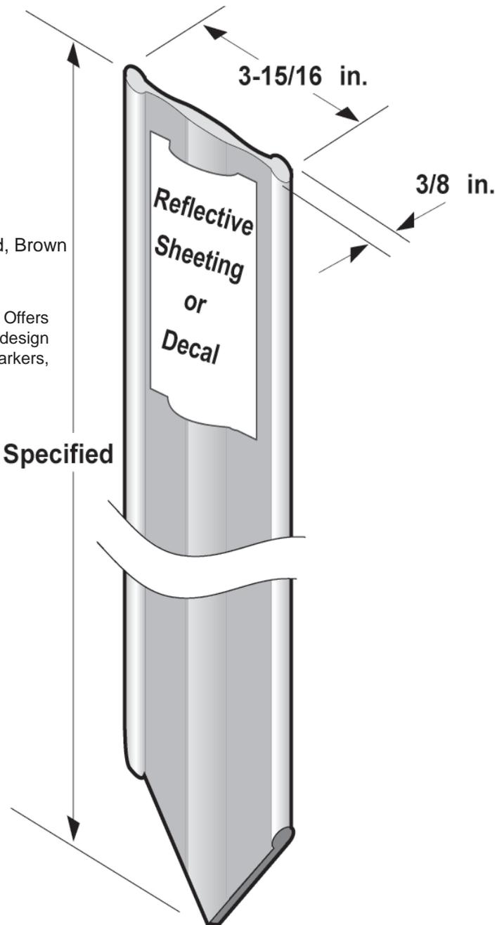
The symmetrical three rib profile optimizes rigidity, stability and flexibility. This provides an unobstructed recessed message area on both sides of the marker, offering protection of the warning message.
